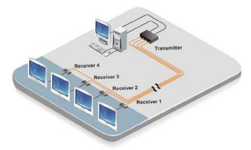
**CrystalView DVI Multi basics** The CrystalView DVI Multi system consists of a transmitter that connects to a PC, server, or KVM switch and up to eight receivers that connect to a remote DVI monitor. The transmitter and receiver units are connected together with up to 220 feet of standard CAT6 shielded cable.
