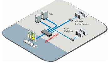
**Models** The QuadraVista Quad Video KVM Switch is available in a single user, four computer model. Adding KVM switches to it can expand the system to 1,000s of computers and serial devices.
