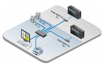
**Models** The QuadraVista 2 Quad Video KVM Switch is available in a single-user, four computer model. Adding KVM switches to it can expand the system to 1,000s of computers and serial devices.
