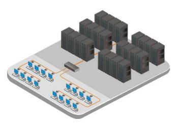
**Cables...** All cabling to the user stations and computers uses standard CATx cable. Max cumulative cable length of 1,000'
