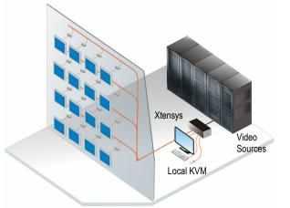
**Cables...** All cabling to the video monitors and video sources uses standard CATx cable. Max cumulative cable length of 1,000'
