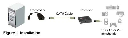
Before you install the CrystalView USB 2.0 CAT5 extender, it is recommended that you pre-plan you system layout, consisting of the placement of the computer, the routing of the CAT5 cabling, and the location of the USB device(s).
