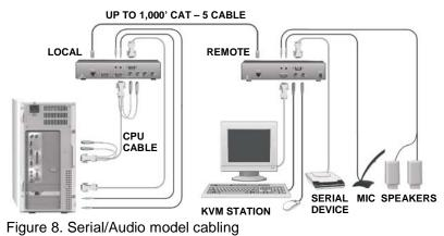
Connect the appropriate CPU cable to the keyboard, video monitor and mouse ports on the CPU. Connect the other end of the CPU cable to the Local Units DB25 connector. Connect the KVM stations keyboard, video monitor and mouse cables to the corresponding connectors on the Remote Unit.
