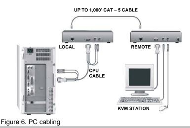
Connect the appropriate CPU cable to the keyboard and video monitor ports on the CPU and to the Local Units keyboard and video monitor connectors. Connect the KVM stations keyboard, and video monitor cables to the corresponding connectors on the Remote Unit.
