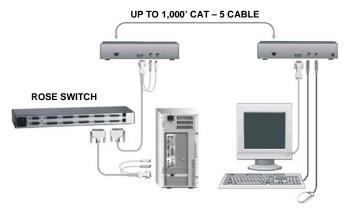
Figure 10. Rose switch cabling
