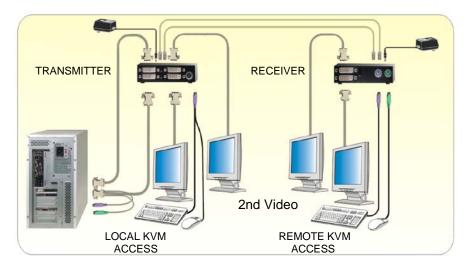
Connect the local USB model transmitter as shown below (single or dual video). A USB hub is used for local keyboard and mouse connections to the computer.
