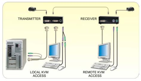
Figure 1. Typical cabling configurations
