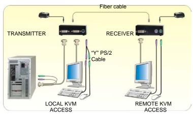
Figure 1. Typical cabling configurations
