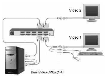
Figure 3. 4U2V Unit installation
