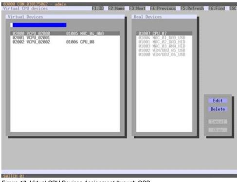
Figure 17. Virtual CPU Devices Assignment through OSD
