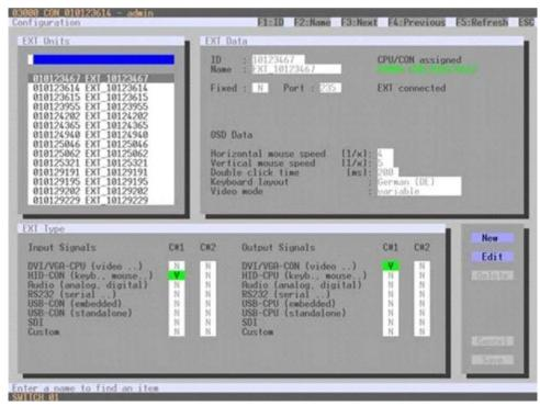
Figure 44. Modifying Mouse and Keyboard Settings through OSD
