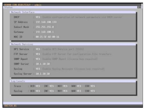
Figure 79. Viewing Network Status through OSD
