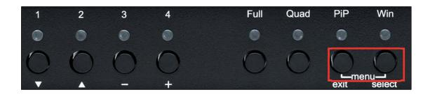
Figure 7. Buttons for Displaying the OSD
