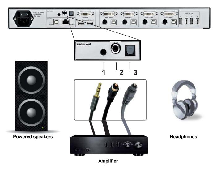
Figure 11. Audio Output Connections
