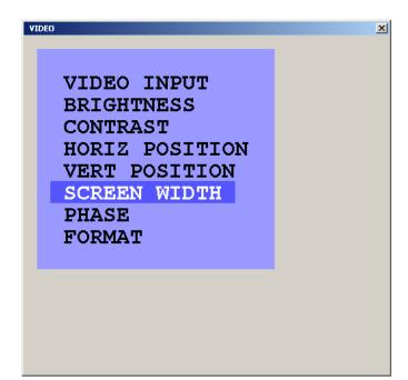
The width of the screen can be adjusted to improve screen quality by selecting the screen width menu, the computer to modify, and adjusting the number of horizontal pixels
