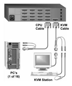
Figure 2. Single Unit configuration
