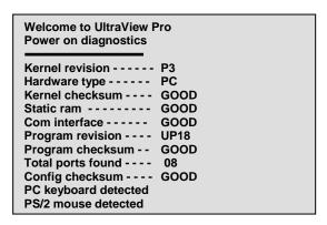
Figure 11. Power-on diagnostic screen
