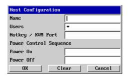
Select each item (1-128) as needed and enter the Name, Users, Hotkey / KVM port keyboard sequence, and power control ON and Off key sequences.
