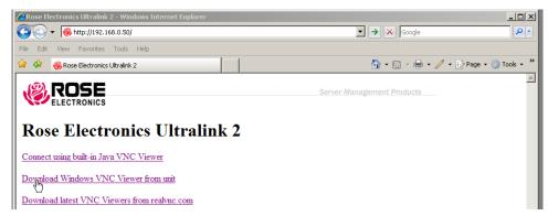
The first time a connection to the UltraView Remote 2 is made, it is recommended that you download the Windows VNC viewer from the unit, save it and run the VNC viewer to connect to the unit directly. Some operating systems may request permission to run or save the program. Save the program to the location wanted and create a desktop ICON for the program. The next time the RealVNC viewer is needed, just click on the desktop ICON to connect.
