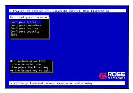
Figure 12. Main configuration menu (Ctrl + F12)
