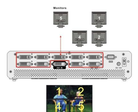
Figure 18. 2x 2 array for VWL-B133FD
