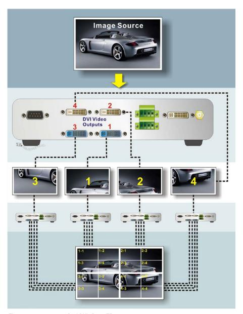
Figure 17. 4 x 4 array for VWL-B122FD
