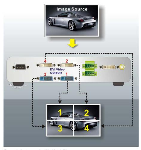
Figure 16. 2 x 2 array for VWL-B-122FD
