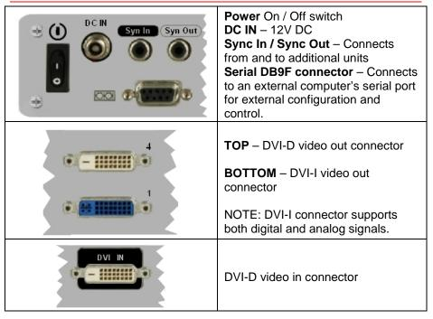
Figure 4. Rear Panel Controls
