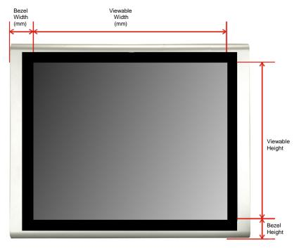
Figure 7. Bezel calculation for VWL-B133FD
