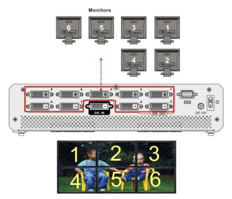
Figure 20. 3 x 2 array for VWL-B133FD
