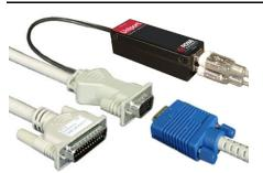
The Uniport "Cable" is a KVM adapter cable. The DB25M connector connects directly to the DB25F KVM port on a Rose KVM switch. The USB connectors and the HD15M connector connect to a KVM stations USB keyboard, mouse and monitor.
