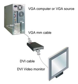
Figure 1. Connectivity Diagram
