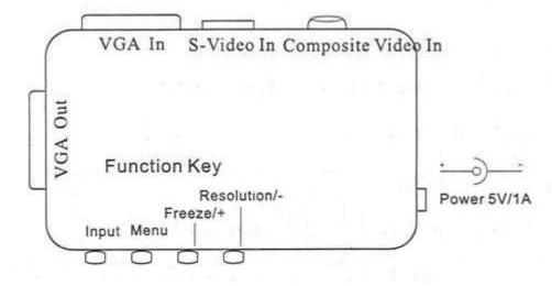
Figure 1. Video Converter buttons and connectors
