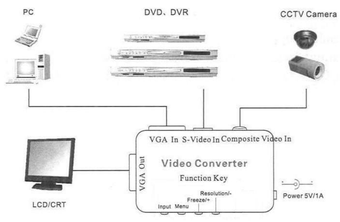
Figure 2. Video Converter Installation Diagram
