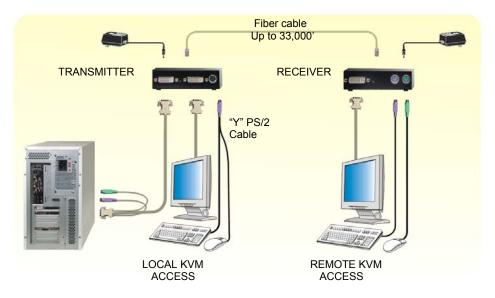
Connect the local USB model transmitter as shown below (single or dual video). A USB hub is used for local keyboard and mouse connections to the computer.
