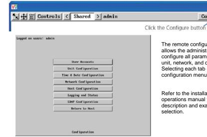
The remote configuration menu allows the administrator to configure all parameters for the unit, network, and other items. Selecting each tab displays that configuration menu.
