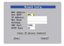
The network information entered should be compatible with the existing network UltraConsole Remote 2 will be installed on. Your network administrator should assign a unique IP address, network mask, and gateway information for the IP Input module.
