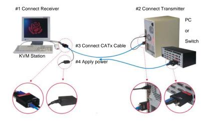
Figure 1. Quick Installation Diagram
